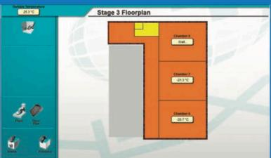
the plant hard during the lower-priced periods, it means that significant financial savings can be made by 'pre-cooling' coldstores prior to periods when a higher tariff applied.
